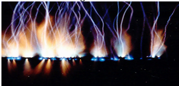
Edge View of Multiple EVO Strikes in Air on an Aluminum Foil Coated with SiC and Epoxy Mix
