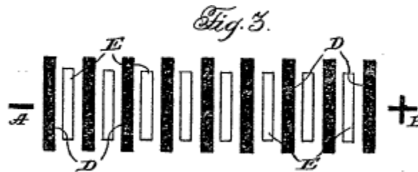
Figure 4 is an elevation of positive and negative electrodes diagrammatically depicted to indicate their relation and use when conveniently placed and disposed within a vacuum tube.
