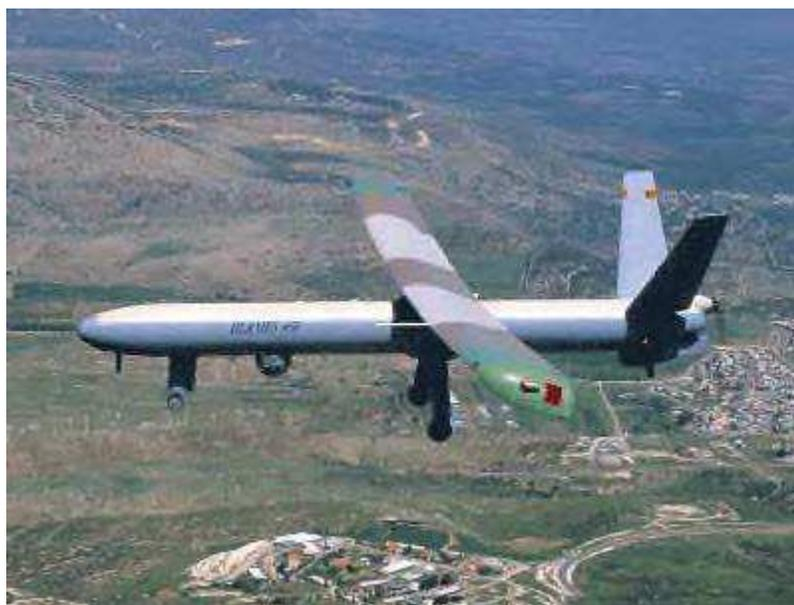
The Hermes 450 is a large, capable 450 kg spy drone manufactured by Elbit Systems of Israel. Able to stay airborne for a maximum of 20 hours, it has a 10.5 metre wingspan and is 6.1 metres long. It can carry a variety of different surveillance packages, including the CoMPASS (Compact Multi-Purpose Advanced Stabilised System), which is a combined laser marker and infrared scanner.
